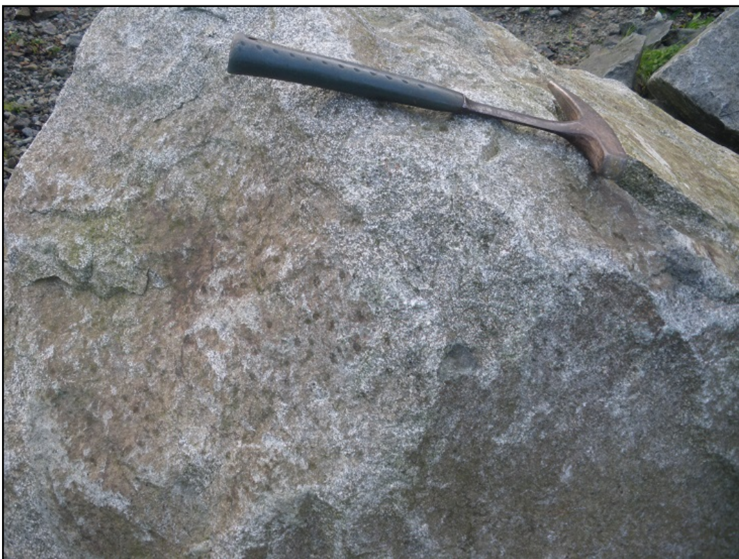
Medium-grained grey-green diorite, typical of rock exposed in the quarry.
